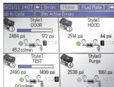
*Control your entire cell with one Advanced Display Module (ADM). Take control of up to four systems with the ADM's easy-to-read system status and alert messages.*
